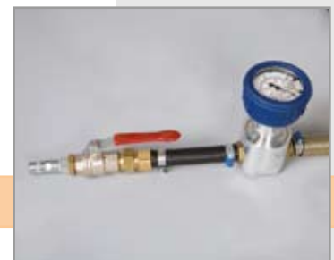
Ball valve with mouth piece and pressure gauge unit with manometer
