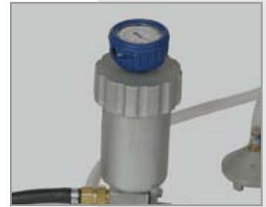
Accumulator with manometer
