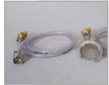
Suction system a) Liquid material b) Mineral-based injection material
